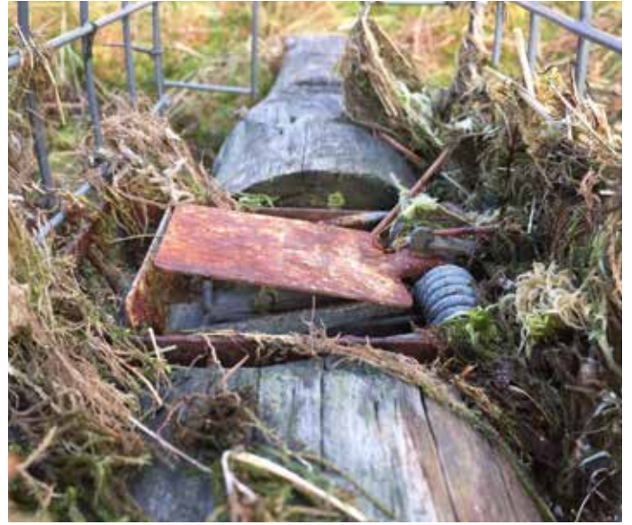
FIGURE 19. Spring traps where vegetation washed down in floods, or the remains of previous captures, has impaired their operating efficiency
