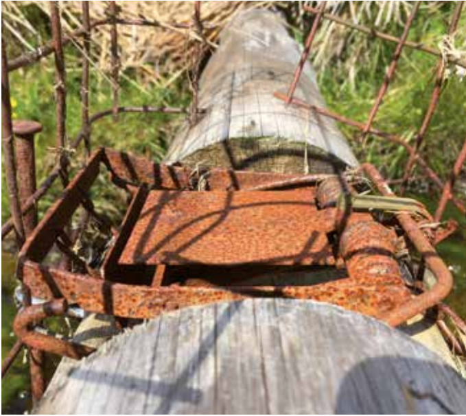
FIGURE 18. Spring traps that have not been maintained and the mechanism has become rusty
