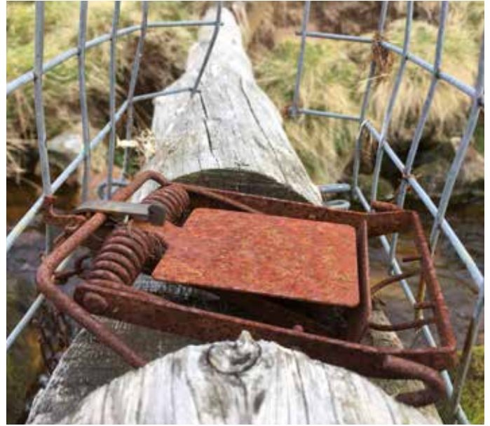
FIGURE 18. Spring traps that have not been maintained and the mechanism has become rusty
